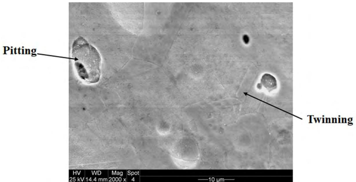
Figure 13. Scanning electron microscope image of UA2015-237-87 copper sheet fragment 2 at 2000x.
