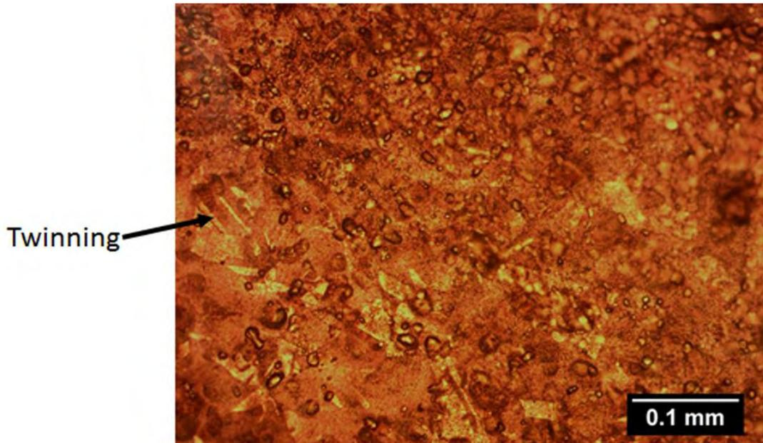
Figure 12. Optical microscope image of UA2016-063-078 (fragment 1) after etching. An equiaxed grain structure is seen as well as annealing twins.
